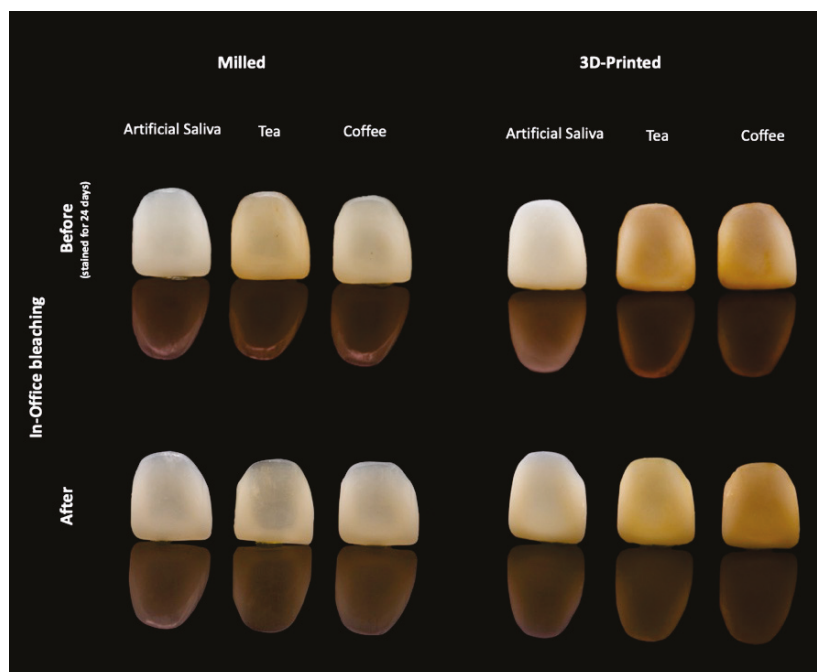
Figure 4. Photograph showing the effect of in-office bleaching in both 3D-printed and milled restoration groups.
