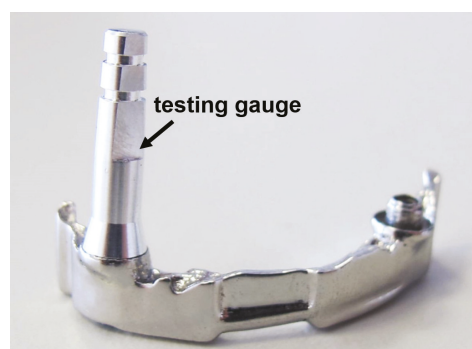
Figure 7. Dental framework with testing gauge.
