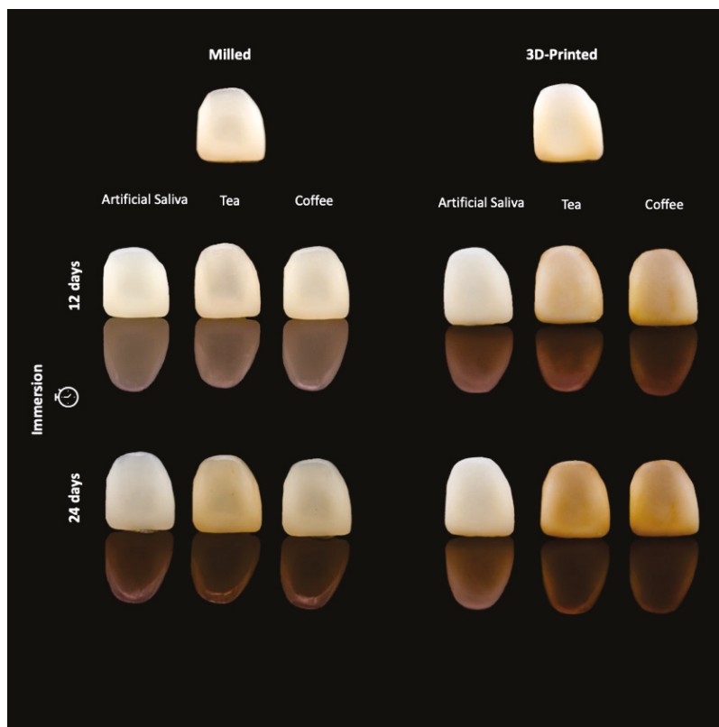
Figure 2. Photograph of \Delta E_{00} of stained milled and 3D-printed specimens after 12 and 24 days of immersion in staining mediums.
