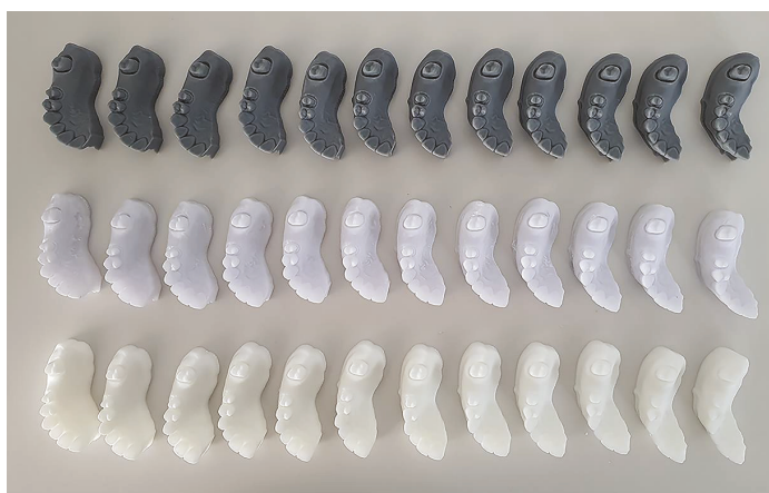
Figure 2. 3D-printed resin models ( n = 36 ) of this study. First row; DLP models, second row; MJP models; third row; SLA models.
