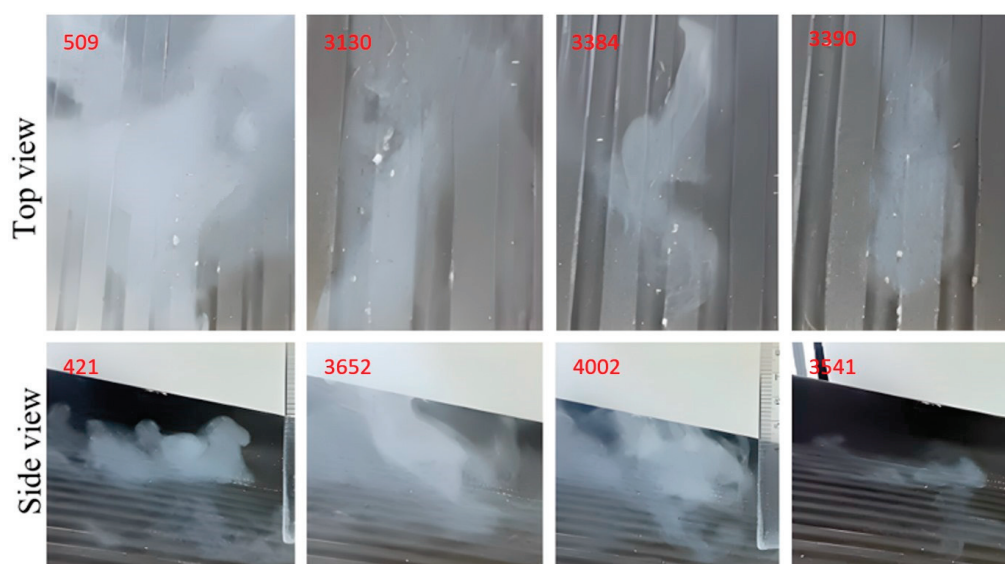
Figure 19. Occurrence of deflagration phenomenon of solid formations obtained after pseudo-desublimation.
