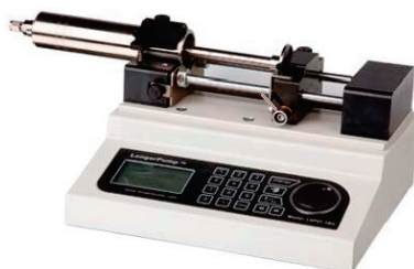
Figure 4. LSP01-1BH injection pump.
