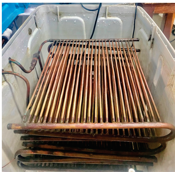
Figure 3. The actual photo of the condenser with eight layers using mini tubes.
