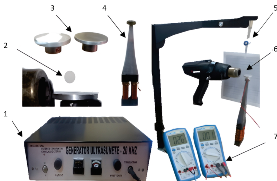
Figure 8. Experimental equipment for the study of AdBlue substance calefaction process.
