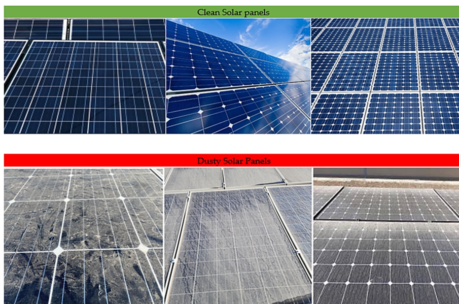
Figure 4. Sample images illustrating clean and dirty PV panels.
