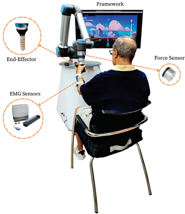
Figure 1. Setup with the robot, EMG sensors, screen, end-effector, and a participant.
