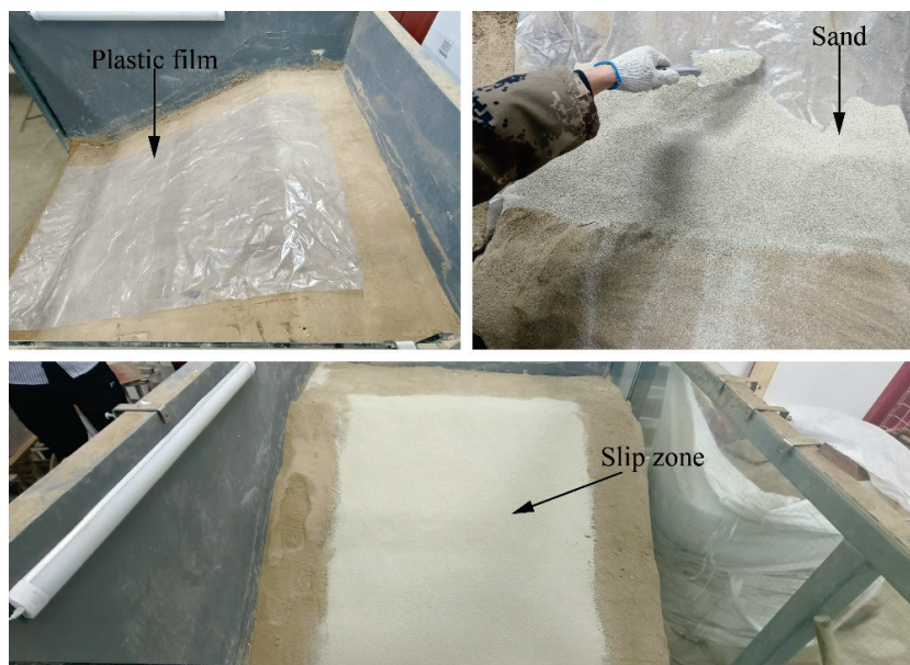
Figure 5. The construction process of the slip zone.
