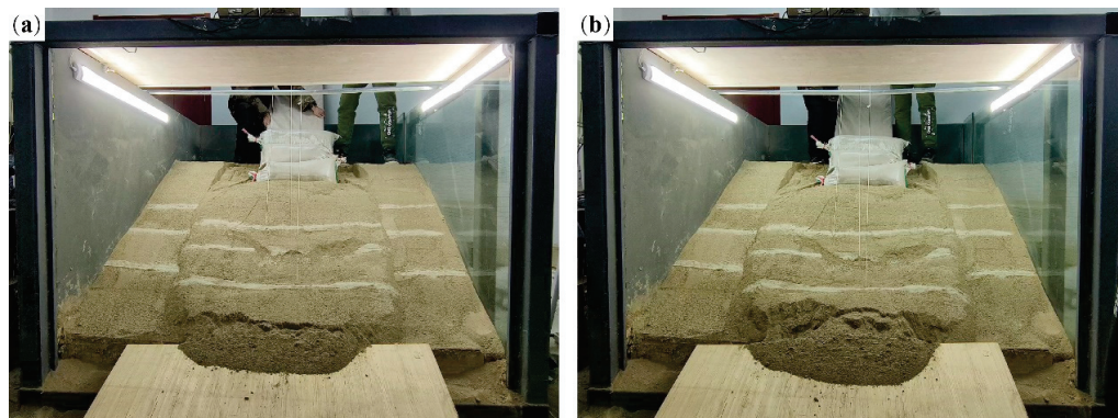
Figure 9. Patterns of crack propagation during the loading process in the Experiment-L: (a) at a surcharge of 90 kg after 4 min and 5 s; (b) at a surcharge of 90 kg after 5 min and 5 s.
