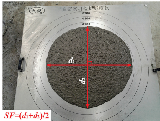
Figure 1. Test and calculation method of slump flow.
