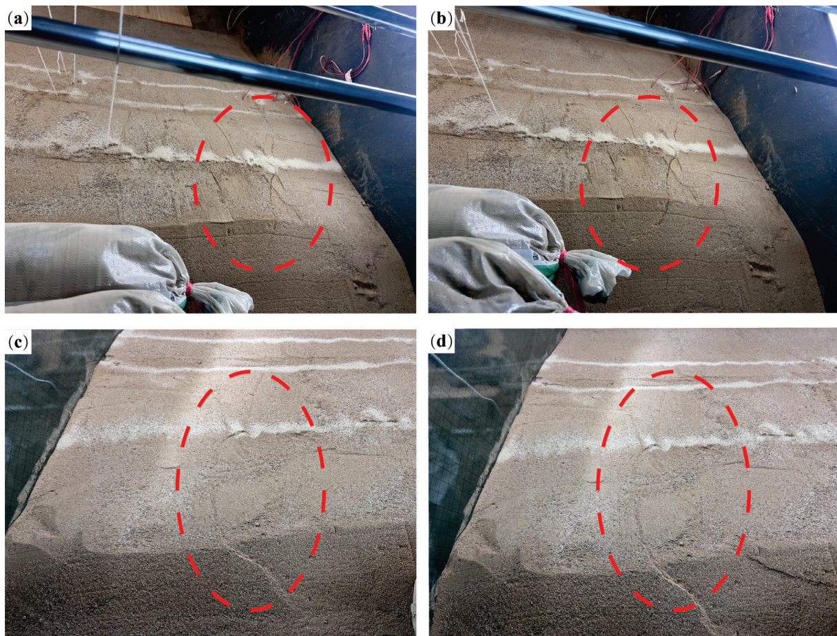
Figure 11. The crack of landslide in the Experiment-LP at a surcharge of 60 kg: (a) the right side after 1 min and 25 s; (b) the right side after 3 min and 55 s; (c) the left side after 1 min and 25 s; (d) the left side after 3 min and 55 s.
