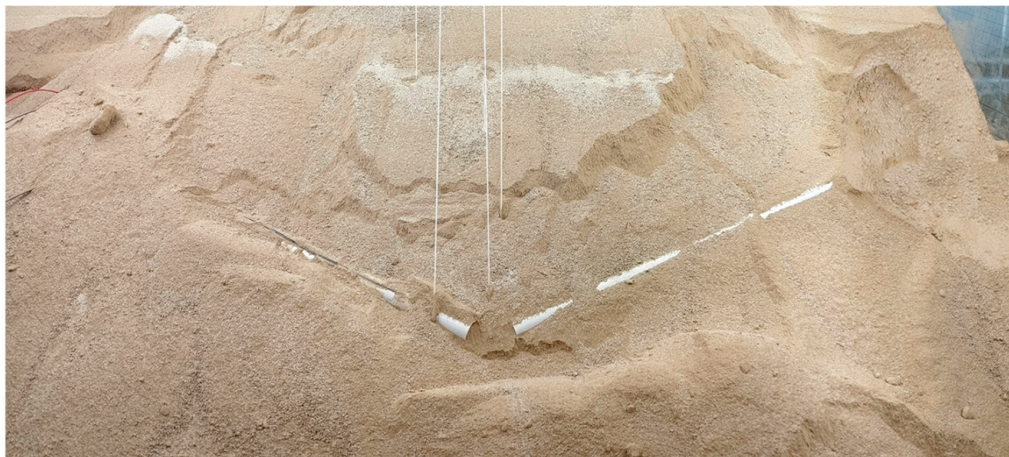
Figure 16. Fracture of the pipeline in the Experiment-LP.
