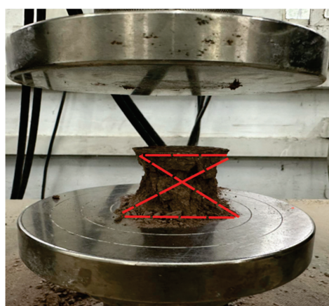
(a) Failure mode of stabilized soil specimen. (b) Curve of unconfined compressive strength with age.
