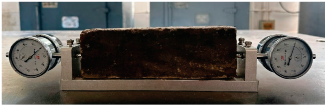
Figure 11. Temperature shrink test specimen.
