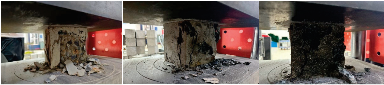
Figure 15. Concrete specimen after uniaxial compressive strength test.
