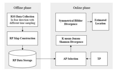
Figure 5. The offline and online stages of location WiFi-based fingerprinting architecture.
