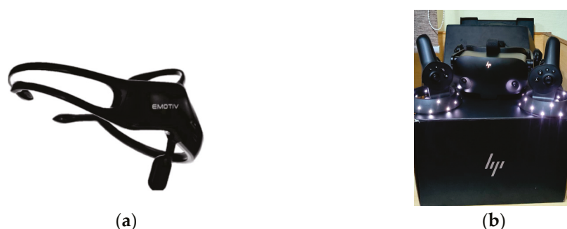
Figure 5. (a). Emotiv 5 Channel EEG. (b). HP Reverb G2 Omnicept HMD. Source: Authors.
