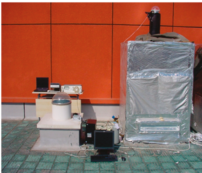
Figure 3. Light pipe-natural ventilation system experimental apparatus.
