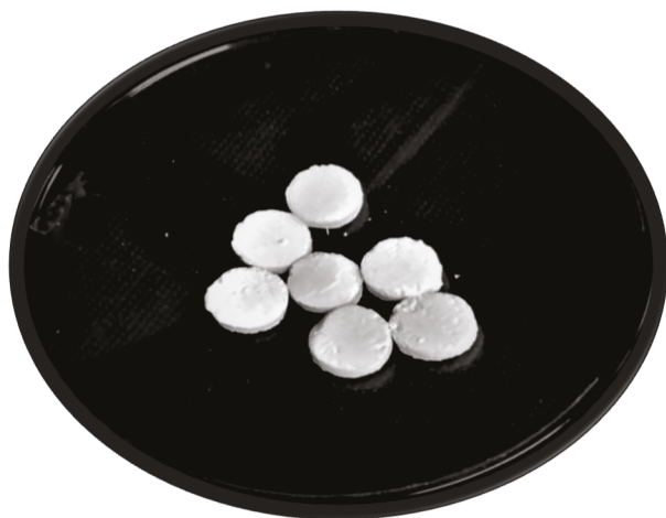
Figure 11. Shaping the sample before immersion in SBF.
