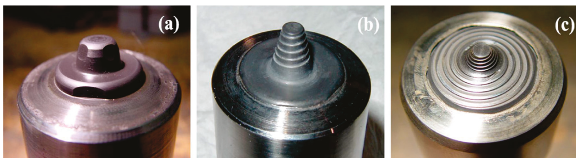
Figure 5. Evolution of the design of PCBN tool: (a) early featureless design, (b) step spiral probe, and (c) convex scrolled shoulder step spiral probe [106].
