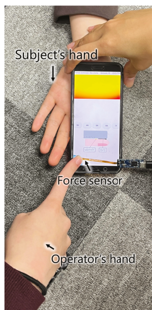
Figure 4. Experimental setup for determining the optimal compression initiation time.
