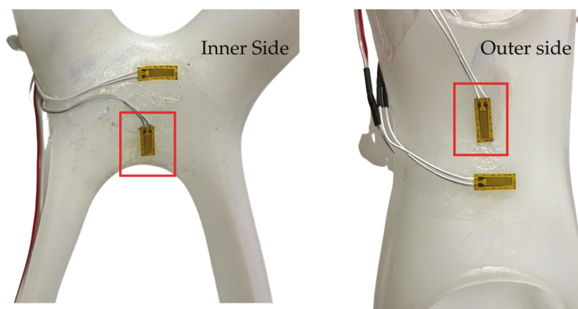
Figure 3. Strain gauges positioning in a full Wheatstone bridge; inside the red square, the longitudinal strain gauges corresponding to a half Wheatstone bridge.
