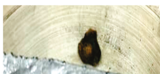
Figure 7. Particle recovered at the end of the cellulose pyrolysis experiment at a target strip temperature of \approx 1000 °C.
