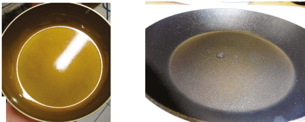
Figure 14. Frying pan metal base with the polyphenolic-TEP binder applied to it ( left ) and finished pan with Teflon applied on the binder according to a proprietary process ( right ) [33].
