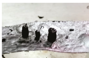
Figure 10. Particle recovered at the end of the naphthalene pitch pyrolysis experiment at a target strip temperature \approx 1600 °C.
