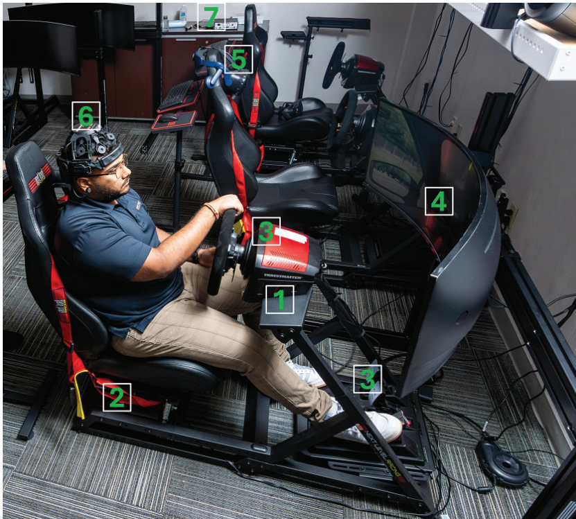
Figure 2. Experimental setup showing a participant operating the multi-participant driving simulator. Key components are labeled as follows: (1) driving cockpit, (2) motion platform, (3) steering wheel and pedals, (4) curved display screen, (5) VR headset, (6) EEG headset, and (7) wireless trigger hub.
