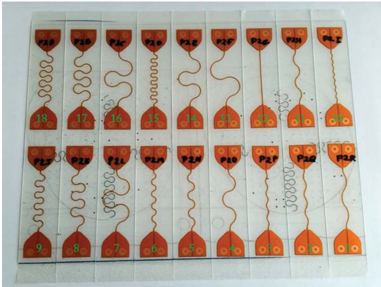
Figure 4. Meander test samples encapsulated in thermoplastic polyurethane using a vacuum press. The black debris visible on the sample originates from FCBs previously cut on the same carrier board.
