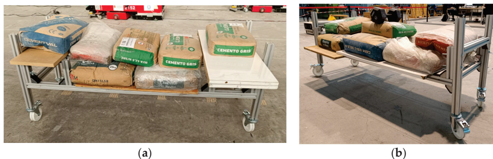
Figure 18. Static load tests on structure: Static Maximum Load Test on Ground-Supported Structure over a short period (24 h) (a); Static Maximum Load Test on Ground-Supported Structure over a large period (20 Days) (b).
