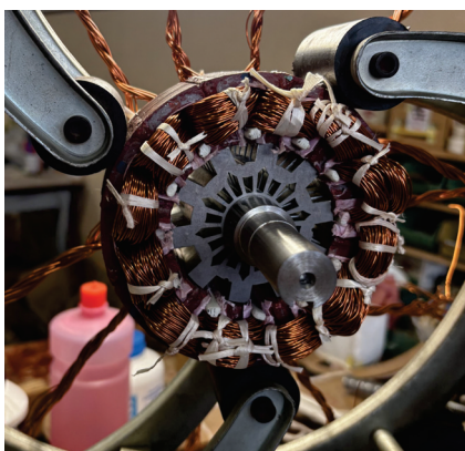
Figure 27. Stator winding process results.
