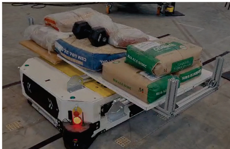
Figure 21. Dynamic Maximum Load Test on AMR-Supported Structure.
