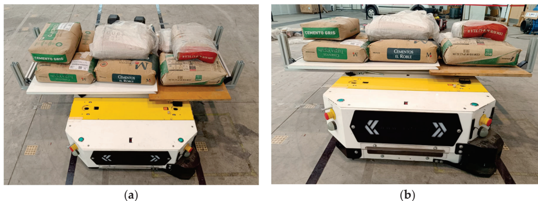
Figure 19. Static load tests on AMR: Static Maximum Load Test on AMR-Supported Structure over Short Term (24 h) (a); Static Maximum Load Test on AMR-Supported Structure over Extended Period (20 Days) (b).
