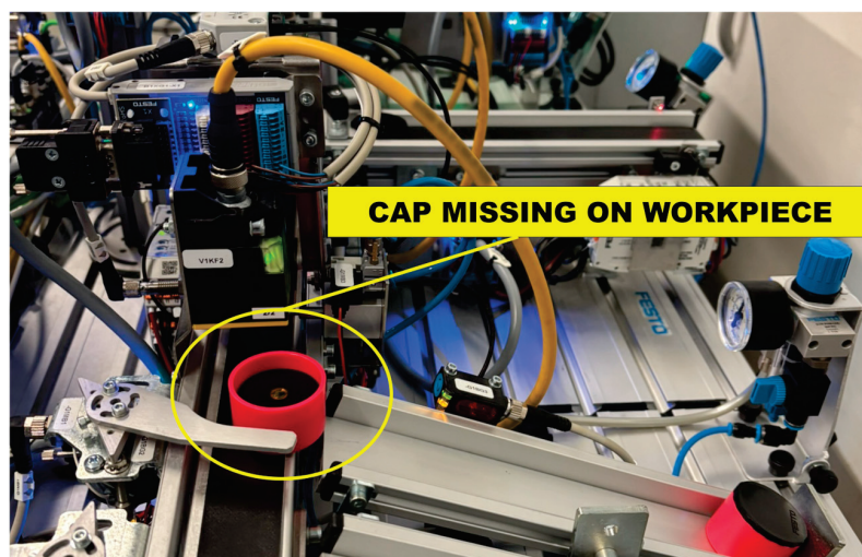
Figure 15. The physical condition of the product during the experimental DDoS attack (scenario 2), documenting the failure to perform the pneumatic operation of deploying the cap in the connection station. The image shows the workpiece without the cap attached due to a communication loss between the PLC control unit and the IO-Link valve terminal, with the control cycle of the production line continuing without immediate detection of this fault at the CPS control or information layer.
