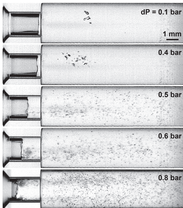
Figure 14. Comparison of downstream bubbles after the start of the decay process.
