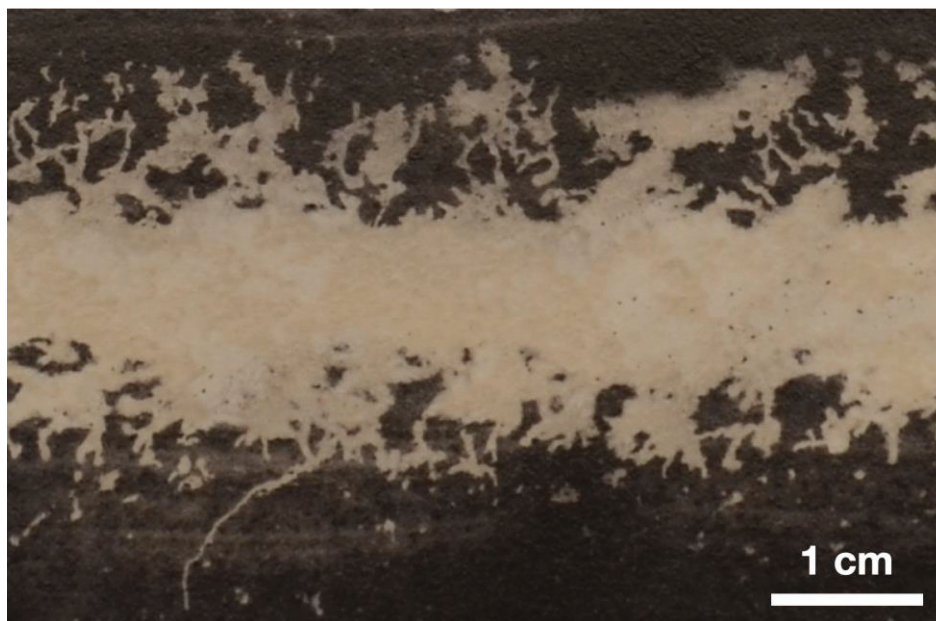
Figure 9. Crack pattern as an ultrasonic transducer with a light mass on the bottom passes by.
