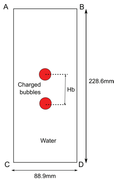
Figure 22. Computational domain setup for the three-dimensional underwater explosion of two bubbles placed vertically in an enclosed region.
