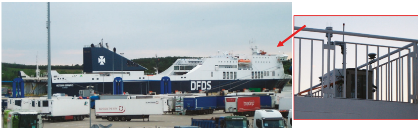
Figure 4. Ship lidar installation on Victoria Seaways—© Fraunhofer IWES.
