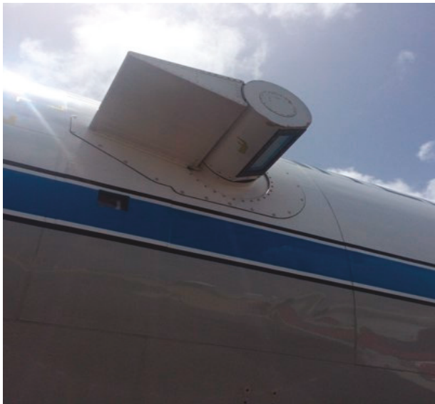
Figure 1. P3 Doppler Wind Lidar (DWL) bi-axis scanner.
