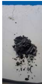
Figure 2. Mg-silicide uncoated after aging at 500 °C for 120 h, in air.
