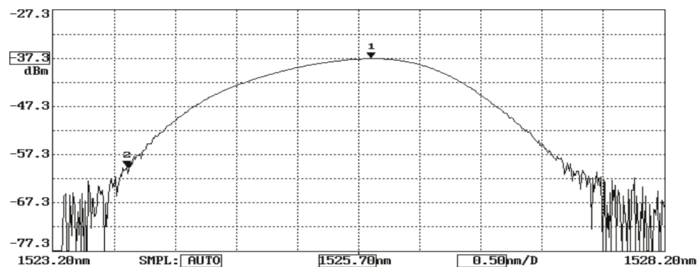
Figure 4. Band pass from the optical filter.
