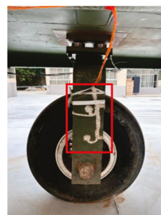
(b) Sensor on the wheel
