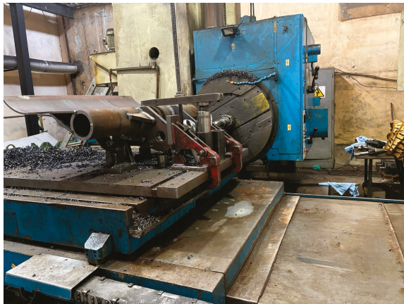
Figure 3. Machining of the mounting holes of the upper part.
