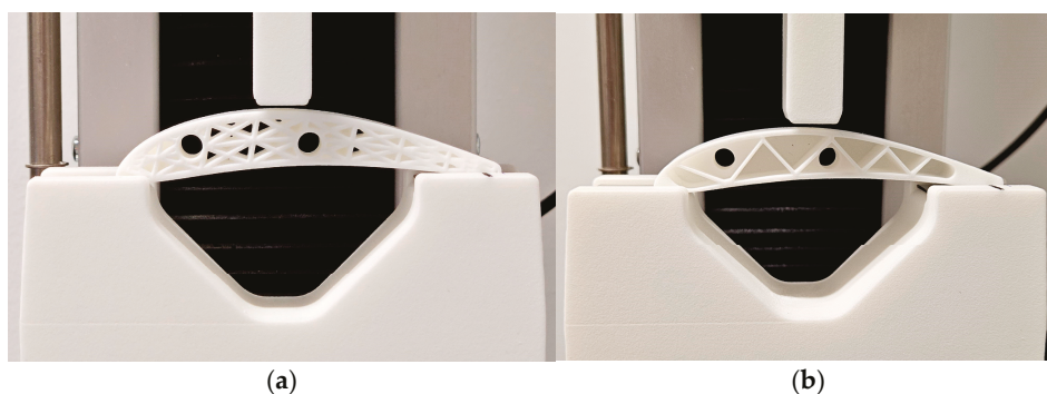
Figure 12. Wing profile insert with different types of internal structures, (a) automatically filled design space with conformal FCCXYZ lattice structure (#3_T4), (b) manually optimized structure (#3_T2).
