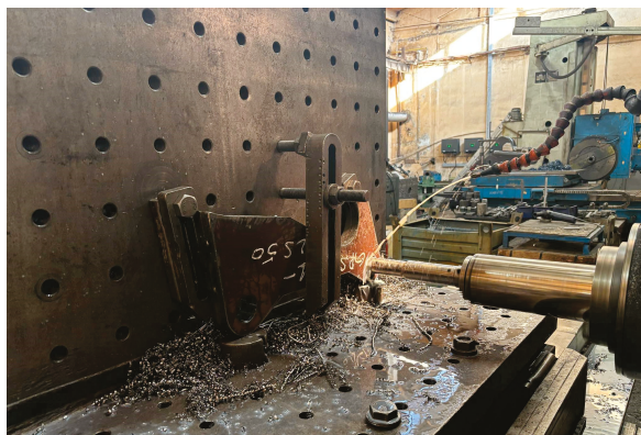
Figure 2. Machining of the ear part from the bucket attachment of the upper part.
