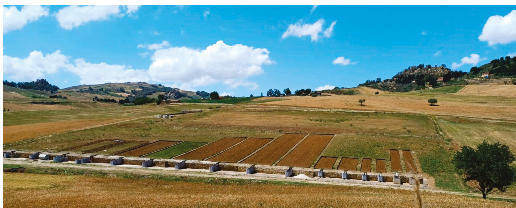
Figure 5. Experimental plots for measuring soil loss at the Sparacia experimental area.
