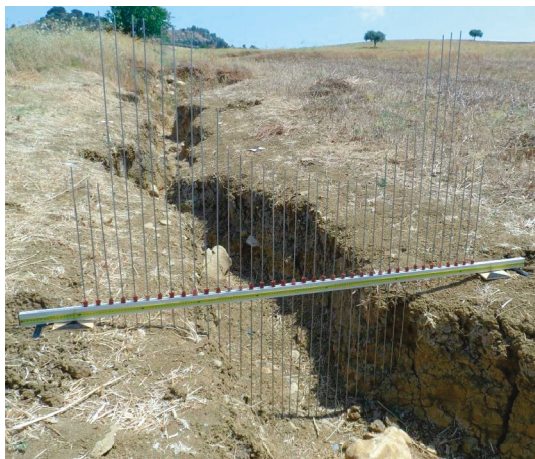
Figure 1. View of a pin profiler (profilometer) (modified from Di Stefano et al. [35]).
