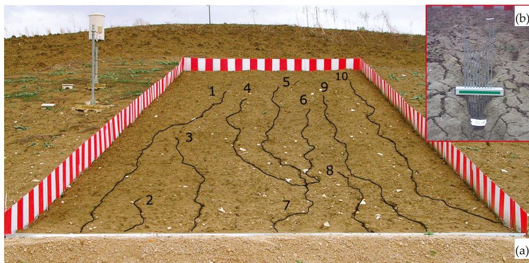
Figure 14. Example of ten rill spatial variability and formation (a) and view of a micro-topographic profiler (b) (modified from [28]).
