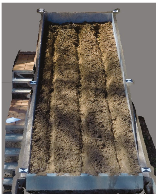
Figure 2. Example of 3D Digital Terrain Model (3D-DTM) of a plot area surveyed for measuring soil erosion (modified from Di Stefano et al. [38]).
