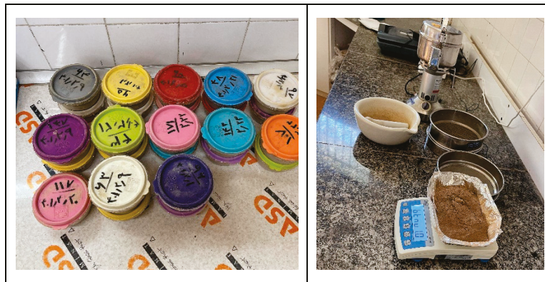
Figure 3. Preparation steps of soil and sediment samples in the laboratory for ^{137}\text{Cs} method.
