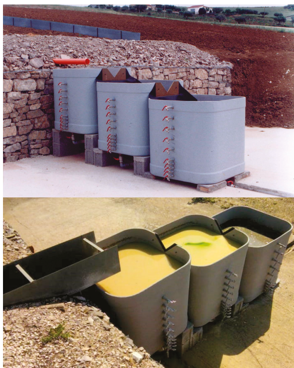
Figure 3. Views of sedimentation tanks used to collect soil loss from a plot.
