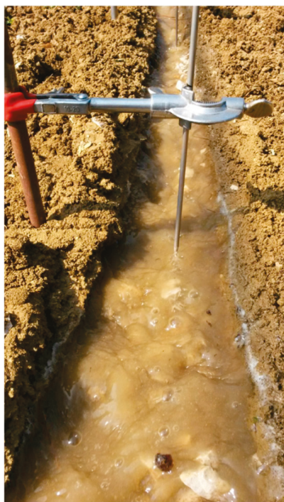
Figure 18. View of point gauges for the measurement of water depth in a rill (modified from Di Stefano et al. [38]).
