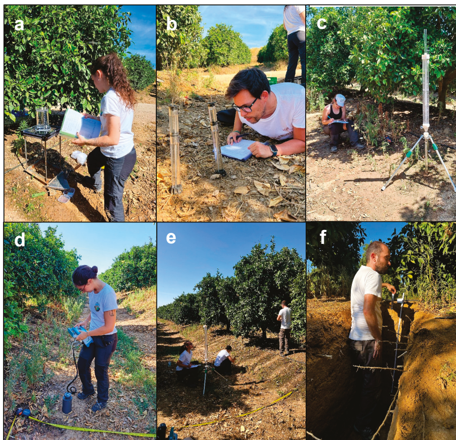
Figure 2. Methods employed in the field experiments and measurements. (a): Rainfall simulations; (b): Infiltration (mini-disc); (c): Guelph permeameter; (d): Soil compaction; (e): CO 2 analysis; (f): soil profile description.
