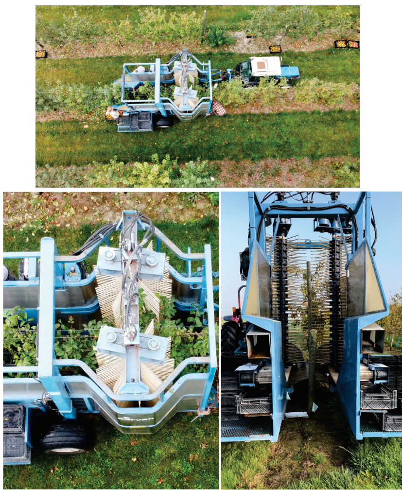
Figure 1. Modified Oxbo-Korvan 930 over-the-row mechanical harvester (Oxbo International Co., Lynden, WA, USA), with two vertical columns with attached, fiberglass harvest rods, during apple harvest in 2023 in Mount Vernon, WA. Photos by Kwabena Sarpong.
