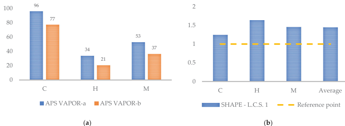
Figure 9. (a) Comparison between actual VAPOR-a and reference VAPOR-b values across different operational modes; (b) normalised SHAPE values for Large Cruise Ship 1. The bars represent the calculated SHAPE for each mode, while the yellow dashed line marks the reference efficiency (SHAPE = 1), indicating that Large Cruise Ship 1 performed less efficiently across all modes.
