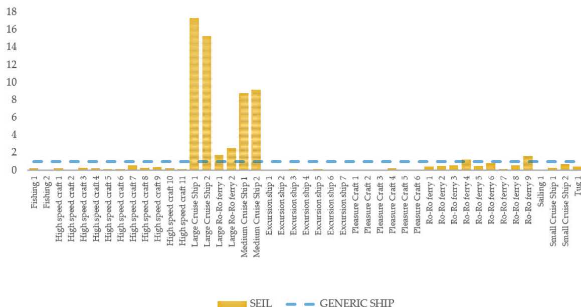
Figure 10. The Ship Emissions Impact Level (SEIL) of vessels calling at the port on the 2nd of July 2019. The SEIL metric expresses the emissions per port visit (voyage) in relation to a standardised “generic ship” represented by the dashed line (value = 1). Notably, the Large Cruise Ship 1 emitted over 17 times the average, while most ships, including Ro-Ro Ferries and High-Speed Crafts, were below or close to the reference point. This visualisation illustrates the significant differences in the impact of emissions between individual ships.
