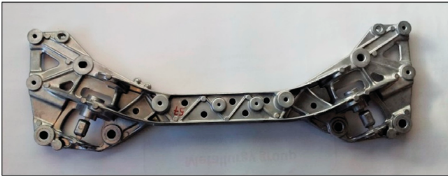
Figure 12. Hollowed aluminum high pressure die casting component.
