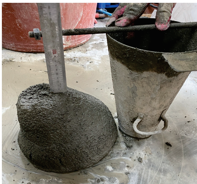
Figure 3. Slump test based on different plasticizer content.
