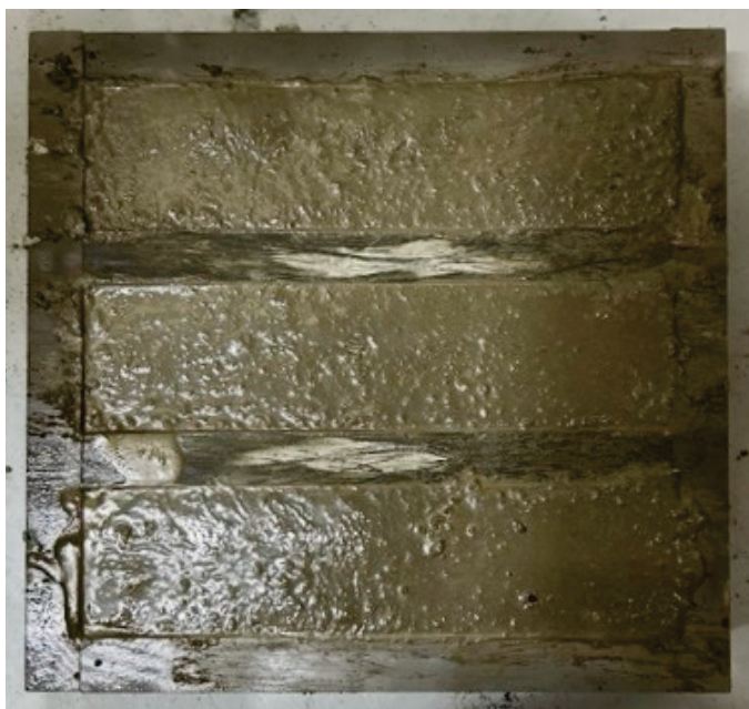
Figure 5. Free drying shrinkage crack test.
