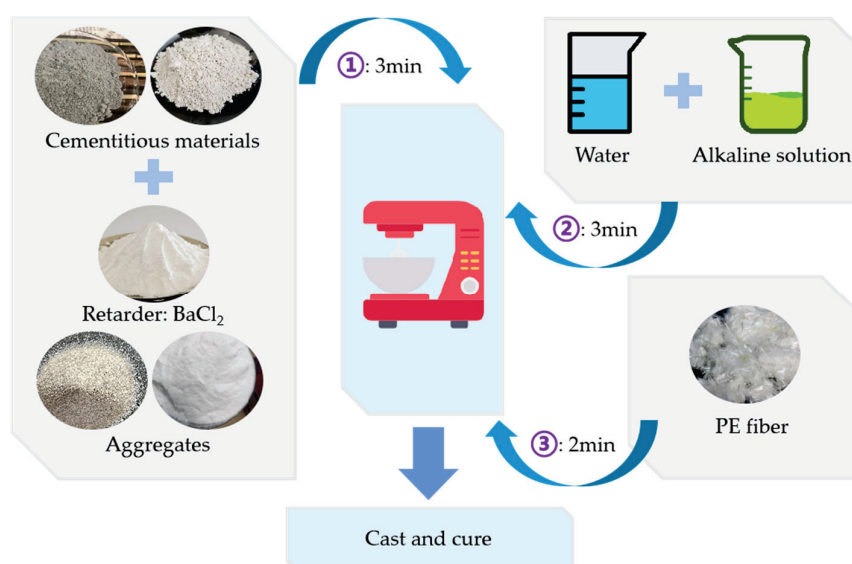
Figure 3. Preparation procedure for P-EHDC.
