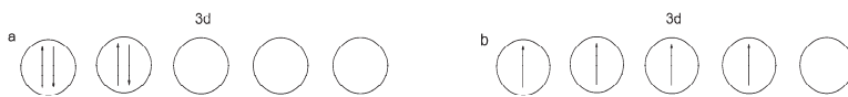
Figure 6. Valence electron diagrams of Cr atom in (a) bulk and (b) monolayer \text{CrSi}_2 systems.
