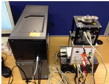
Figure 5. Quanser SRV02 servo based unit.
