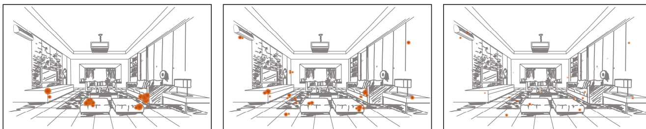
(b) Process of pathogen spread via surface touch — the infection risk first increases and then decreases.
