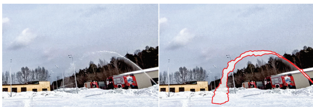
Figure 10. Fragments of the fire-extinguishing agent jet image from the fire monitor after preliminary processing (left) and boundary extraction (right).
