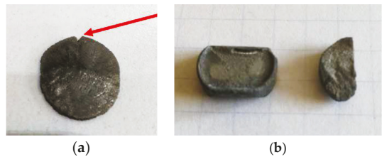
Figure 18. Titanium samples sintered by AC and tested by (a) compression with the red arrow identifying a fracture and (b) indirect tensile testing. The sample in (a) has a relative density of 71% and the samples in (b) have relative densities >80% (left) and <80% (right) with corresponding ductile and brittle behaviour, respectively.
