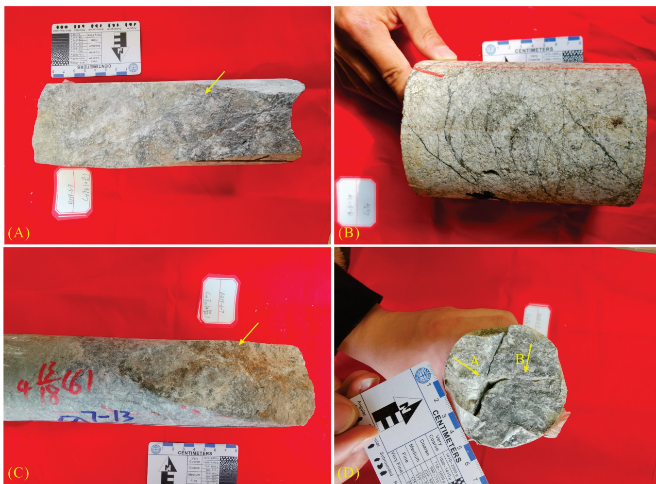
Figure 6. Tectonic fracture characteristics in cores of metamorphic rocks from the Bozhong depression, Bohai Bay Basin. (A) High-angle fractures from Well B19-7 at a depth of 4683.21 m; fracture surfaces are uneven. (B) Fractures from Well B19-14 at a depth of 4362.46 cm; tectonic fractures intersect to form a network of fracture systems. (C) High-angle fractures from Well B19-7 at a depth of 4625.56 m; fracture surfaces are uneven. (D) Tectonic fractures from Well B19-7 at a depth of 4682.22 m; later fractures in Group B terminate earlier fractures in Group A.
