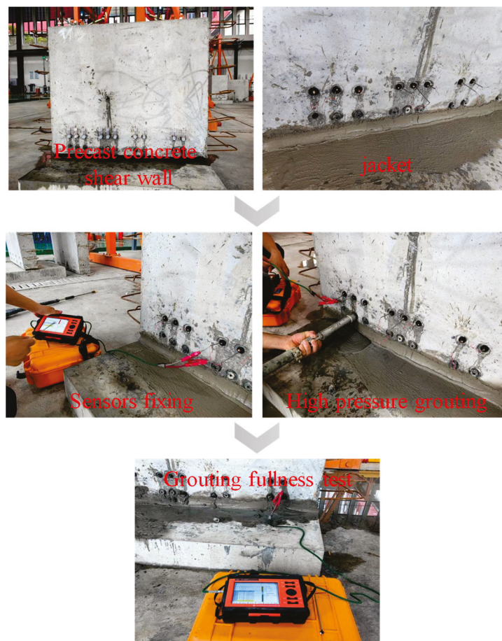
Figure 6. Schematic diagram of field demonstration.
