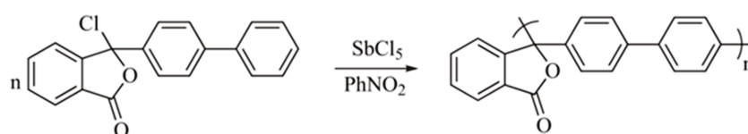
Figure 2. Poly(diphenylene phthalide) C4 synthesis scheme.
