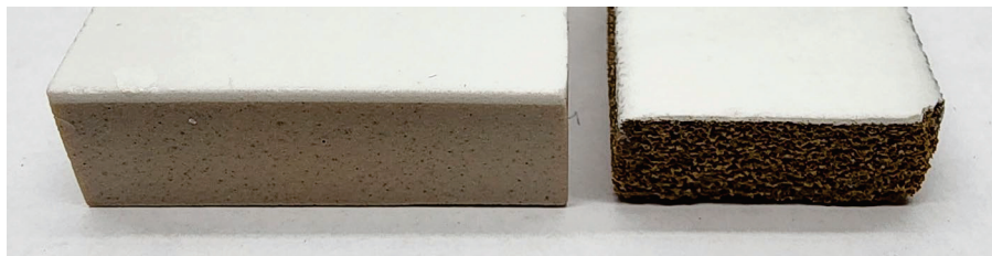
Figure 11. (left) Standard glazed sanitaryware part, (right) part printed with SA18, engobed and glazed.
