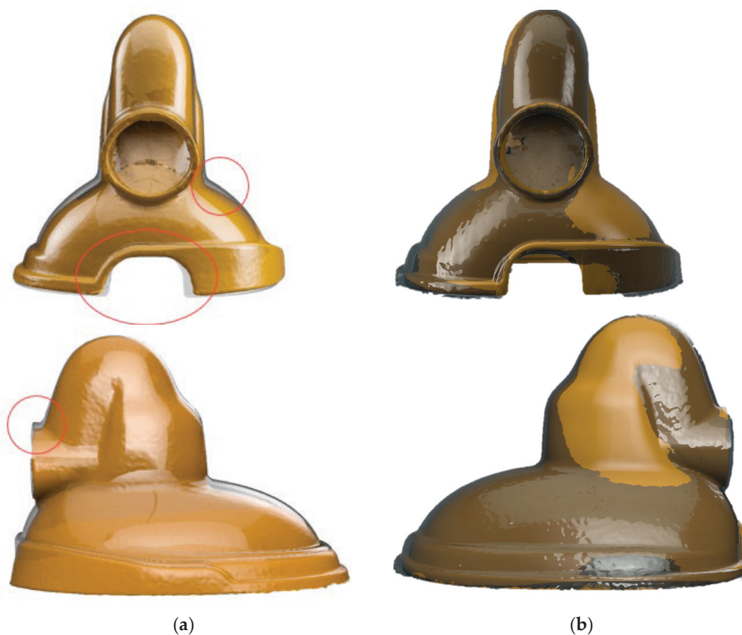
Figure 8. Comparison of the scanned printed part (yellow) vs. the original model (transparent): (a) first try-outs, (b) SA18 printed part. The red circle highlights the shape differences.
