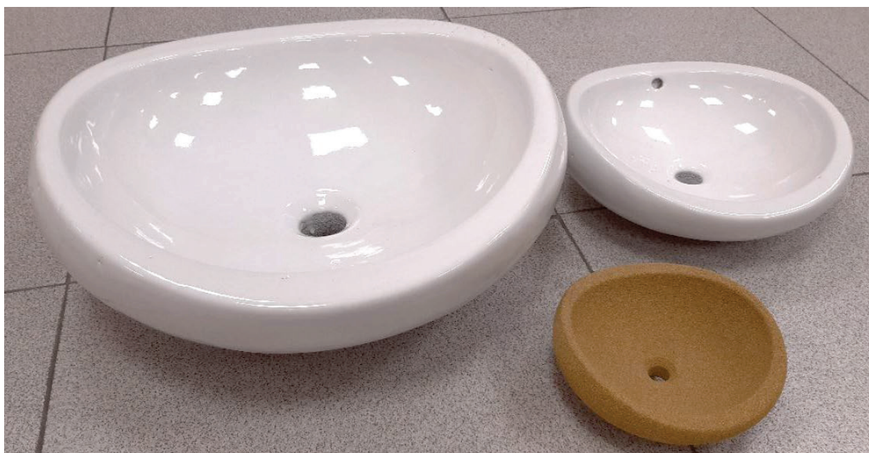
Figure 12. Different printed and sintered washbasins. Top left: real-scale glazed washbasin; top right: scaled, glazed washbasin; bottom right: scaled sintered washbasin.
