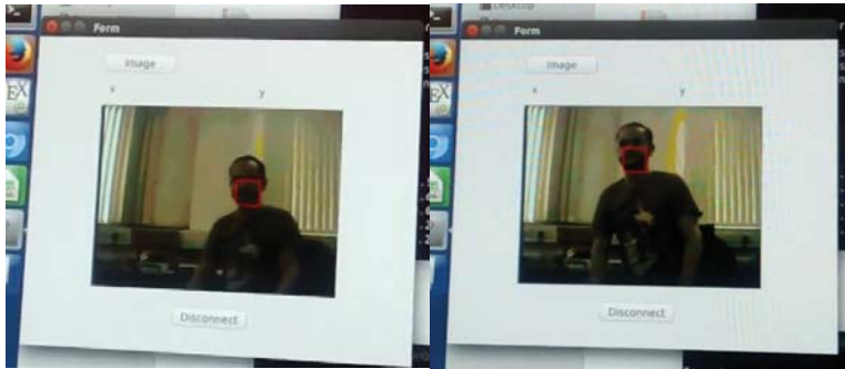
Figure 15. MeanShift Tracking: real-time face tracking displayed on PC. Image sent from Zedboard over Ethernet connection.
