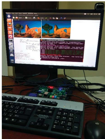
Figure 11. Hardware–software co-design implemented on the Zedboard FPGA platform.
