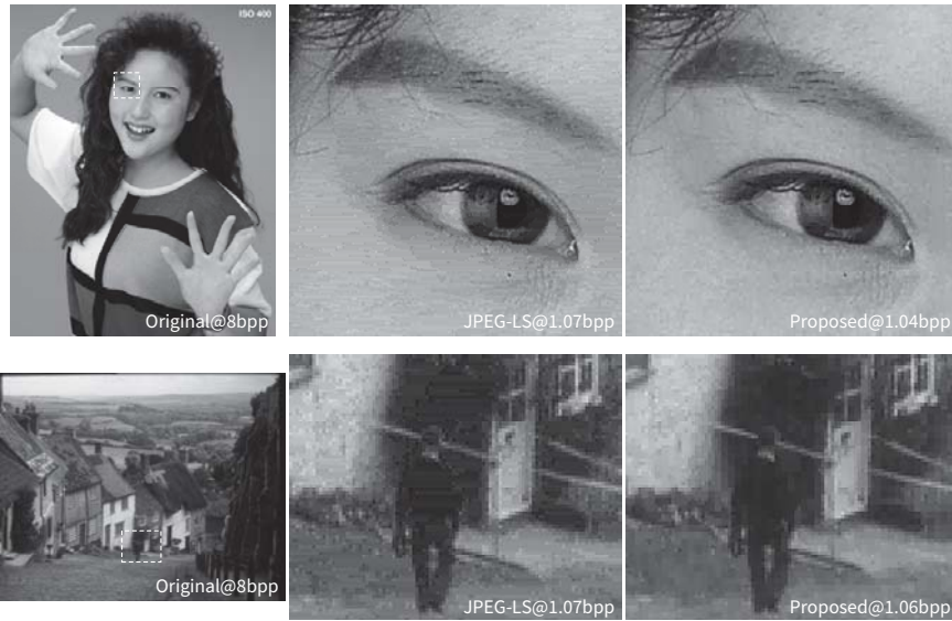
Figure 26. Visual quality of images compressed by JPEG-LS and the proposed JND-based perceptual codec at closely comparable bit rates: top and bottom, WOMAN and GOLD image; and left to right, original image, selected section compressed by JPEG-LS, and same section compressed by the perceptual codec.
