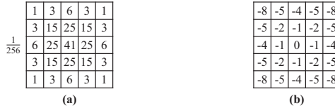
Figure 21. Coefficients for the sample filters used for testing in experiments 1 and 2. (a): FIR filter; (b): morphological filter structuring element offsets.
