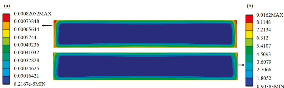
Figure 8. Equivalent stress and strain distribution cloud diagram of the SL before optimization.
