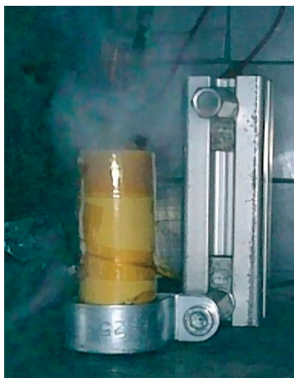
Figure A3. LFP cell during CH experiment at ca. 928 s after beginning of the experiment.
