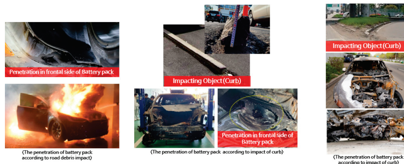
Figure 3. Damage shapes of vehicle structures and battery packs in post-collision fires from direct impacts to the battery pack located at the bottom of EVs. (Yellow cycle is battery impact point).
