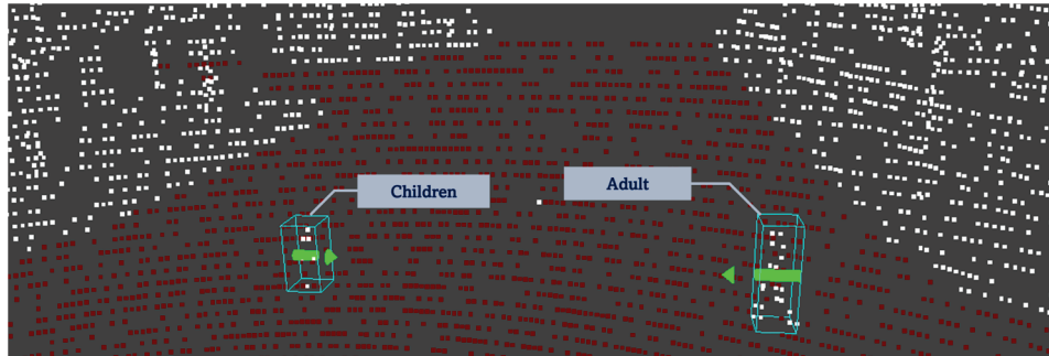
Figure 21. Pedestrian data captured by a 64-channel LiDAR (intersection).
