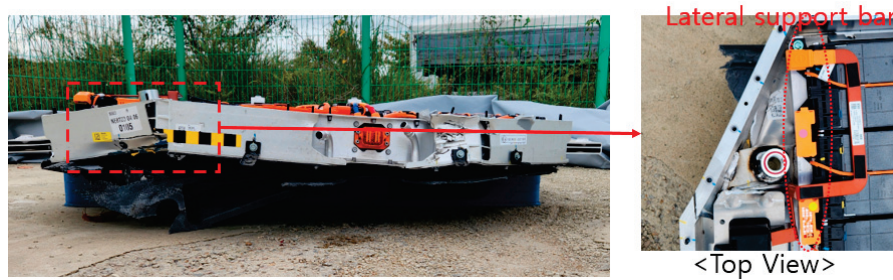
Figure 18. Excessive damage to the front face and internal frame of the battery packs following 30 km/h trolley test using a square impactor.
