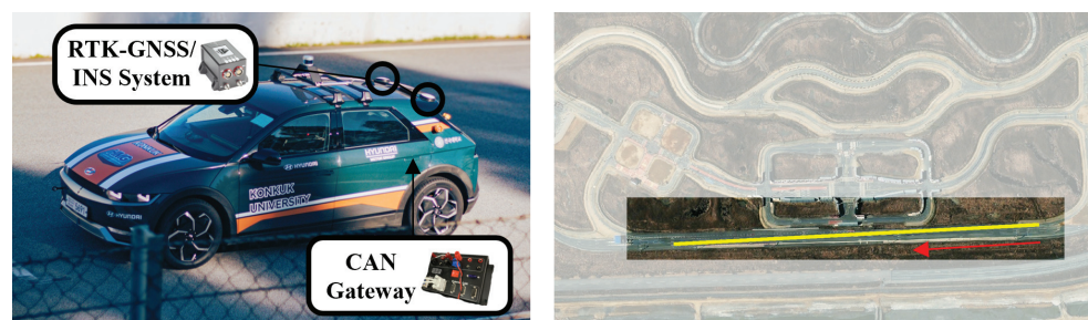
Figure 9. Experimental AEV Platform, Hyundai IONIQ5, and the test site, K-City highway section.
