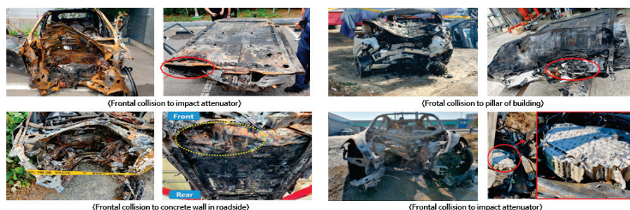
Figure 2. Damage shapes of vehicle structures and battery packs in post-collision fires following high-speed frontal collisions in EVs. (Red and yellow cycles are battery impact points).
