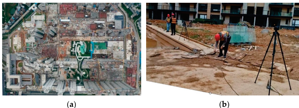
Figure 7. Photos of site measurement at a similar depot: (a) an aerial photo of the TOD and (b) noise and vibration measurement devices on the ground of the TOD.
