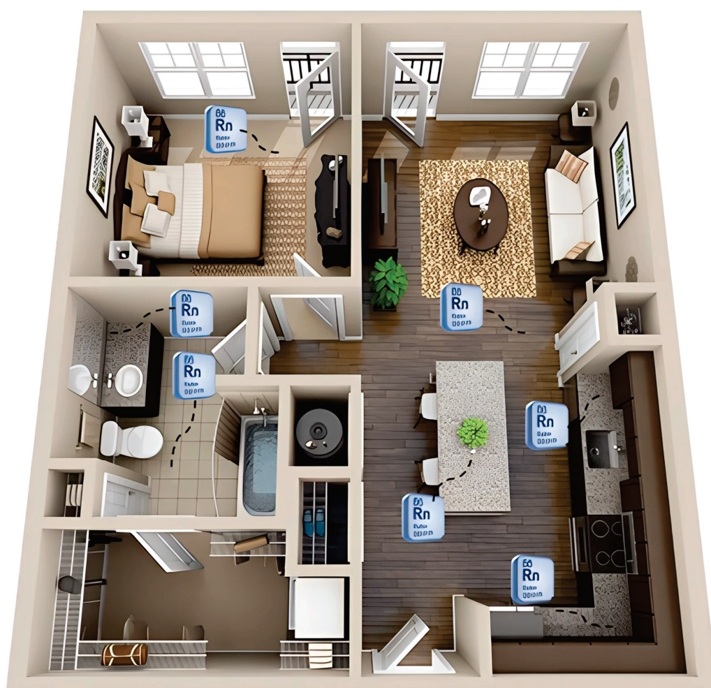
Figure 2. Schematic model for the visualization of radon and thoron emission and the sources of radioactive gases and gamma radiation (including kitchen worktops, kitchen island, floor, tiles, and hand basin top) within a one-bedroom house. In this instance, the effective volume is estimated at 121.6 \text{ m}^3 , with stone (e.g., granite, limestone and sandstone) coverage ranging from 42 to 80 \text{ m}^2 .
