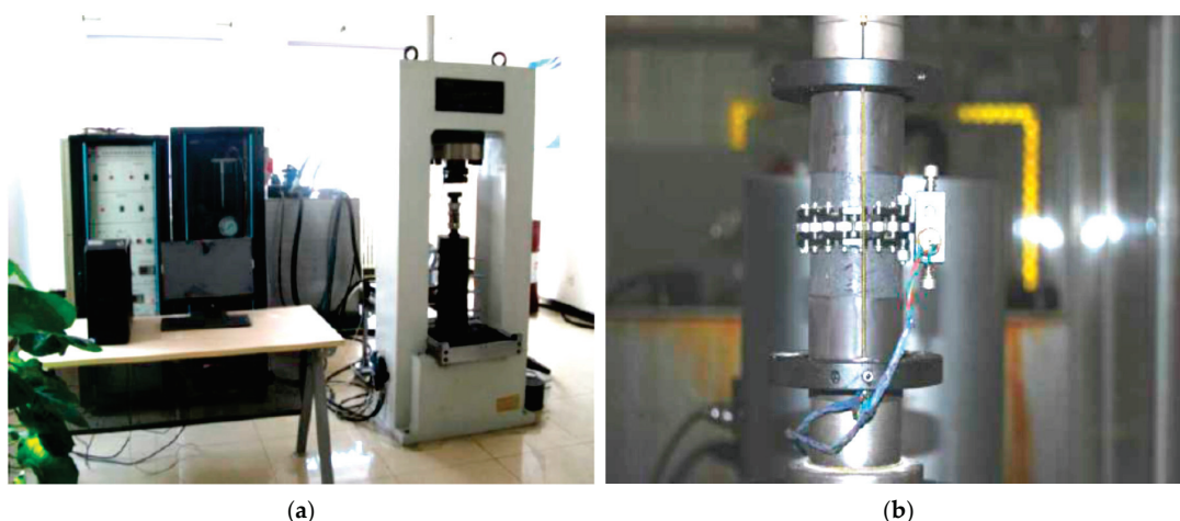
Figure 1. Main test equipment: (a) TAW-2000 electro-hydraulic servo testing machine; (b) LVDT displacement sensor.
