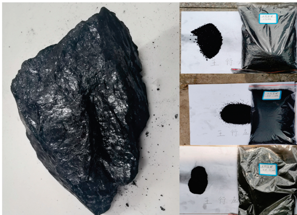
Figure 1. Mesoscopic characteristics of the coal sample.
