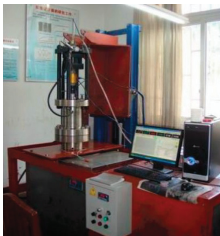
Figure 3. Gas-bearing coal thermal fluid–solid coupled triaxial servo test system.
