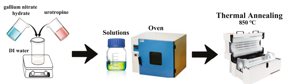
Figure 1. Schematic diagram of the synthesis process of the 1D porous \beta -Ga 2 O 3 nanorods.
