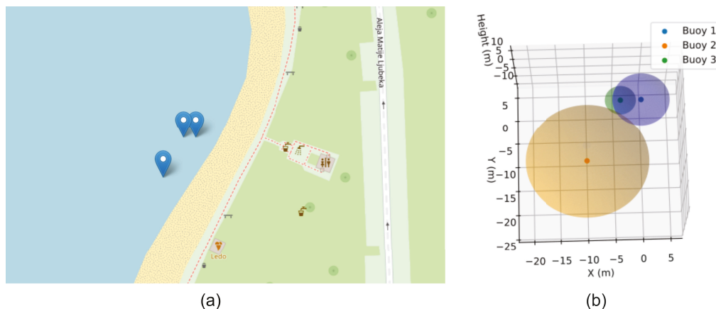
Figure 6. The trilateration algorithm used for underwater localisation provides accurate spatial mapping of buoys and UAEs, enhancing the platform's capacity to precisely track assets in submerged environments. Location of the buoys (a). Data processed using the trilateration algorithm (b).
