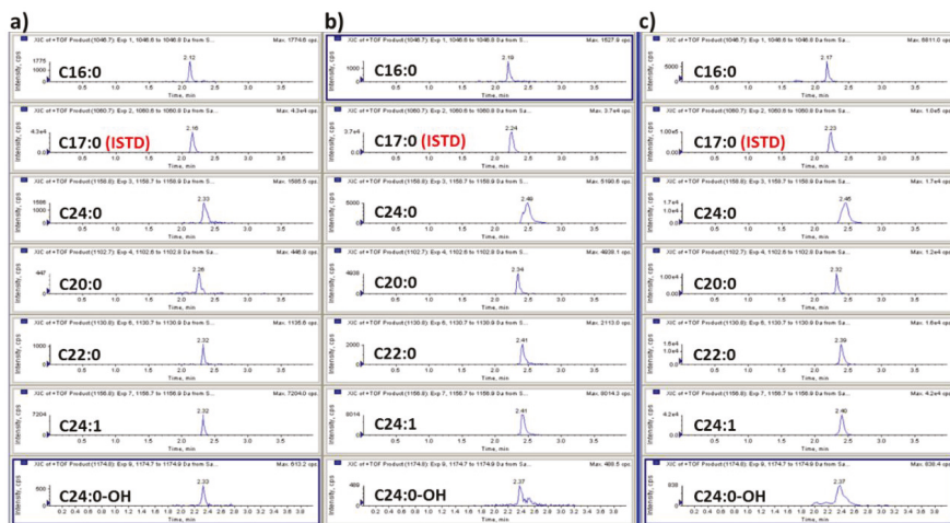
Figure 7. LC-MS chromatograms of GB3 in (a) plasma; (b) heart; and (c) spleen from the Fabry disease model mouse.
