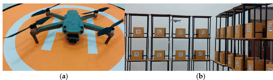
Figure 17. Experimental setup. (a) Scanning UAV (DJI Air 2S) with a three-axis gimbal camera on the take-off/landing pad. (b) Indoor mock-warehouse testbed with parallel racks and QR-tagged cartons arranged on three levels for inventory scan trials.
