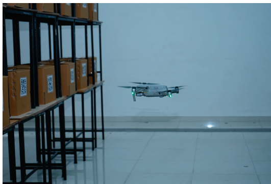
Figure 18. Single-UAV flight during rack scanning (experimental setup). The DJI Air 2S hovers mid-aisle while reading front-facing QR codes affixed to cartons at three shelf levels.
