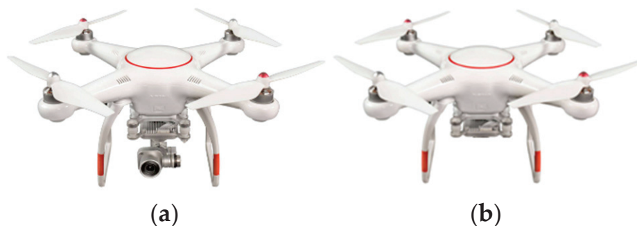
Figure 2. Visual presentation of the “DJI Phantom” drone: (a) with a camera, (b) with the camera removed for the drone’s side circuit needs.
