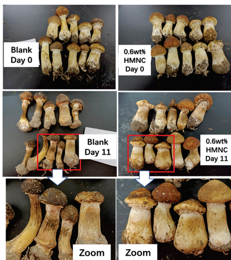
Figure 6. The freshness preservation evaluation of Agaricus mushrooms using commercial PE film and PBAT-HMNC (PBAT-HMNC-0.6).
