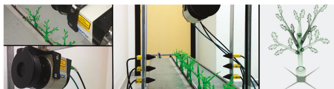
Figure 1. Details of the sensors on the laboratory platform (vertical LiDAR and Light-beam sensors) for the detection and structure of the modular 3D plant.
