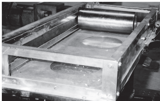
Figure 6. The build chamber showing a thin layer of powder presented as a single layer on a planar surface prior to direct photonic interaction.
