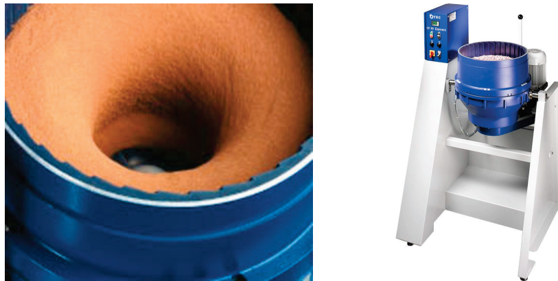
Figure 1. Centrifugal disc machine principle (LJMU).
