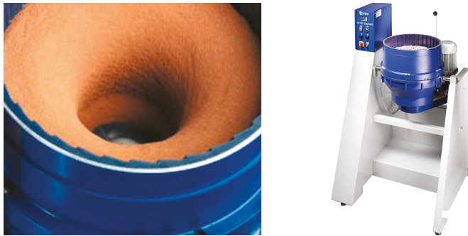
Figure 1. Centrifugal disc machine principle (LJMU).
