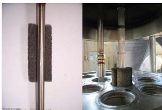
Figure 5. R-02 reactor catalyst arrangement.
